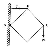
As shown in the figure, a square uniform lamina of weight W is hinged to a vertical wall at A with its plane vertical. Another body of weight W is suspended from the opposite corner C. The lamina is supported with its diagonal AC horizontal by means of a horizontal string joining B to the wall. The tension T in the string is
