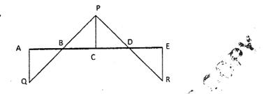
The bending moment diagram of a samply supported beam, supported at both ends is shown in the figure. In that case, which of the following figures shows the nature of shear force distribution in the beam? It is given that AB = BC = CD = DE and |AQ| = |PC| = |ER|.
