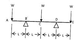
A uniform simply supported beam is loaded as shown in the figure. Which of the diagrams below best represents its bending moment distribution?
